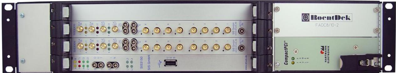
*Figures: **RoentDek fADC8** module (here **fADC8/10-2**) with two 10 bit ADC units, e.g. for readout of up to two **RoentDek HEX**anode detectors (here with SMA inputs. LEMO 00 option is also available).*
