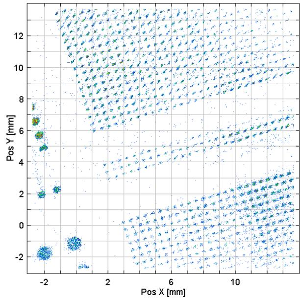
Figure: Position picture acquired with a **RoentDek** HEX75-detector. Fast Xenon ions are projected through a pin hole mask. The position resolution in this plot is better than  $100 \mu\text{m}$  FWHM (data acquired at  $2.5\text{Gs/s}$ ,  $1.25\text{Gs/s}$  typically result in  $130 \mu\text{m}$ ).
