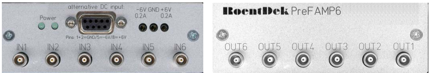
Figure 3: rear panel of PreFAMP6 (left) with signal inputs and DC power input via 9-pin sub-D connector or 2mm pins. Right: front panel of PreFAMP6 with signal outputs.
