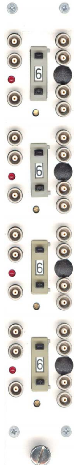
Figure: front panel of LogX4. The range selector switch is behind the black cover
