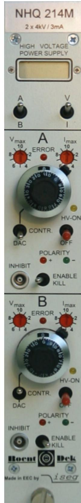
Figure: 2x4kV high-voltage power supply (front panel)
