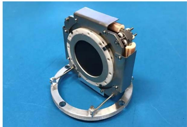
Mounting schemes for high anode/holder potentials  $> 5$  kV (**XHV**) require the use of ceramic distance pieces beyond the metal rods. **RoentDek** can provide such mounting schemes for at least up to 10 kV potential as add-on to any of the above-described options.
