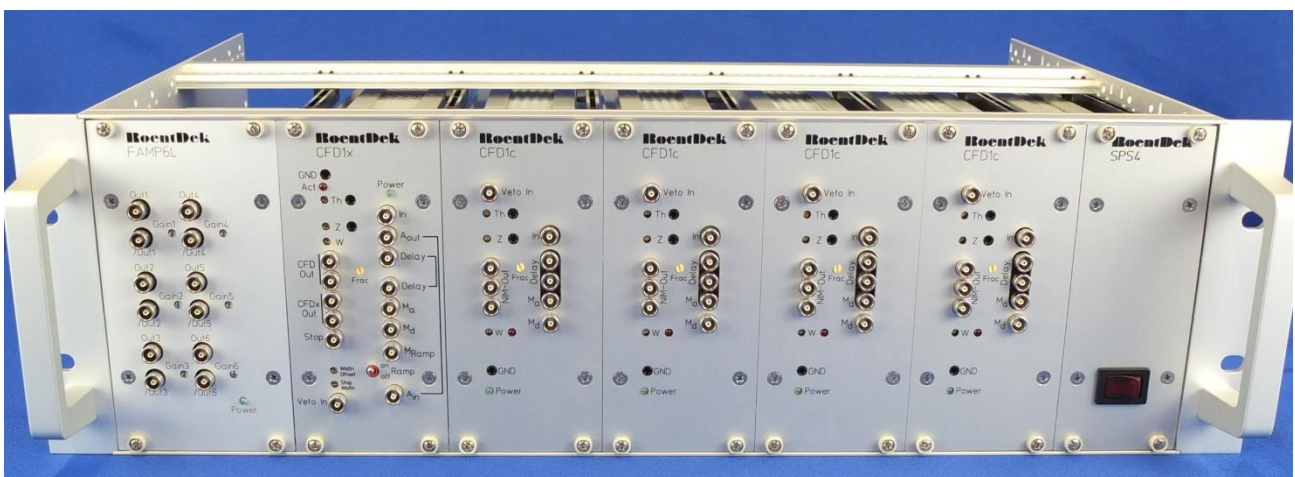
Figure 1: FEE5x with 19" 3HU crate hosting six amplifier channels (FAMP6L or two FAMP3) and 4+1 CFD channels (four CFD1c plus one CFD1x). The CFD1x has additional circuits to transform pulse height information into a time delay for recording by a TDC channel. Below: version FEE5 with CFD4L (replacing four CFD1c) and standard CFD1c (can also be upgraded to FEE5x). RoentDek can also provide a FAMP6 and CFD4c as NIM cassette units and a frame for CFD1c/CFD1x for mounting in a NIM bin (not included). For cabling please refer to the FEE5 connection scheme .
