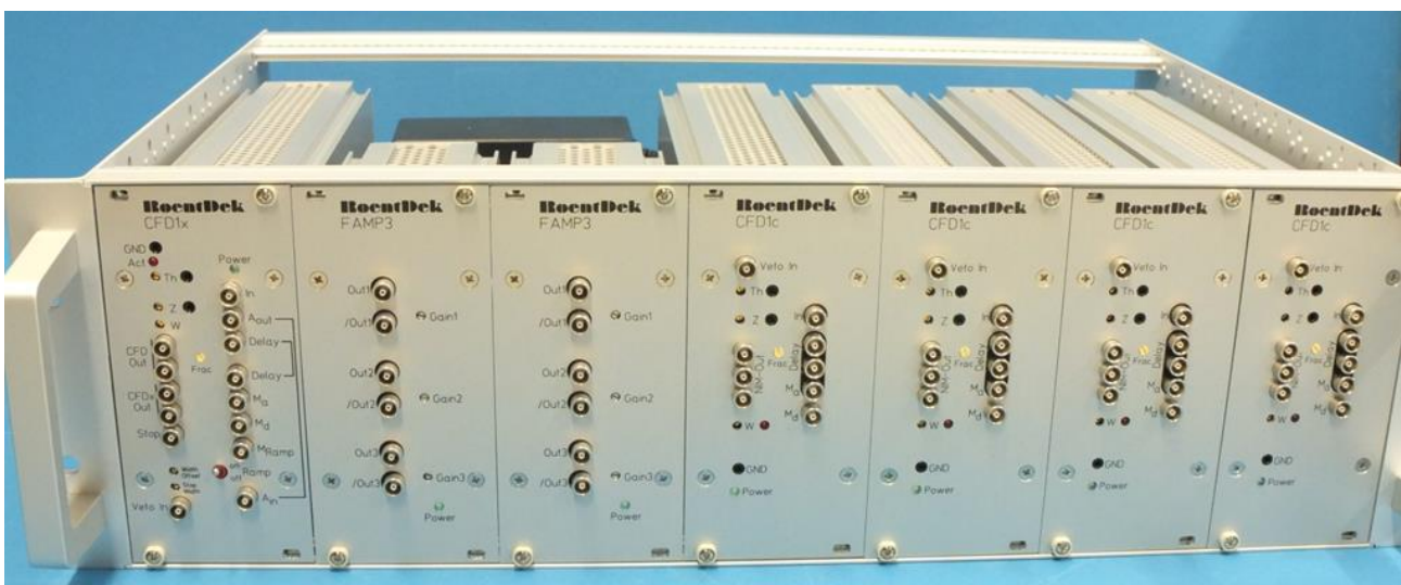
Figure 1: FEE5x with 19" 3HU crate hosting six amplifier channels (two FAMP3) and 4+1 CFD channels (four CFD1c plus one CFD1x). The CFD1x has additional circuits to transform pulse height information into a time delay for parallel recording on a TDC channel. Optionally, RoentDek can also provide a CFD4c (NIM cassette) which replaces the four of CFD1c units on the right (no crates are provided if this combination is chosen).
