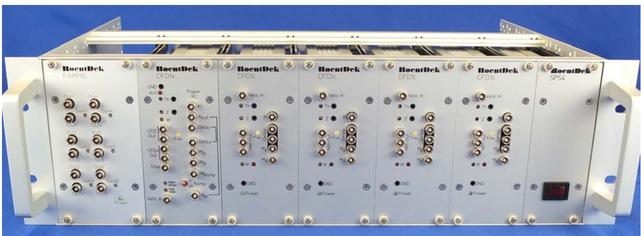
Figure 1: FEE5x with 19" 3HU crate hosting six amplifier channels (FAM6L or two FAMP3) and 4+1 CFD channels (four CFD1c plus one CFD1x). The CFD1x has additional circuits to transform pulse height information into a time delay for recording by a TDC channel. RoentDek can also provide a CFD4c (NIM cassette) which replaces the four of CFD1c units on the right (no crates are provided if this combination is chosen).
