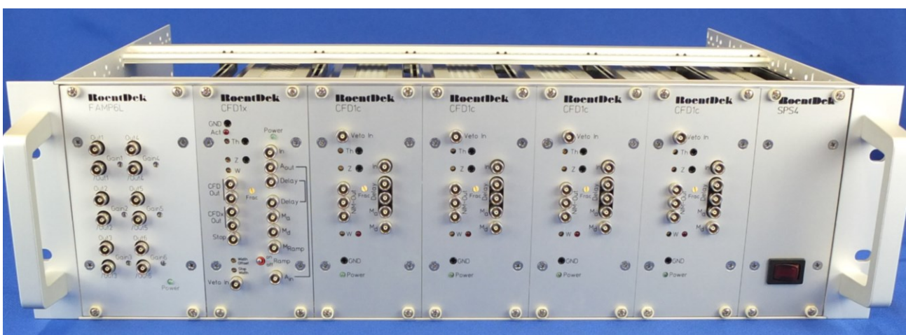
Figure 1: FEE5x with 19" 3HU crate hosting six amplifier channels (FAM6L or two FAMP3) and 4+1 CFD channels (four CFD1c plus one CFD1x). The CFD1x has additional circuits to transform pulse height information into a time delay for recording by a TDC channel. RoentDek can also provide a CFD4c (NIM cassette) which replaces the four of CFD1c units on the right (no crates are provided if this combination is chosen). For cabling please refer to the FEE5 connection scheme .
