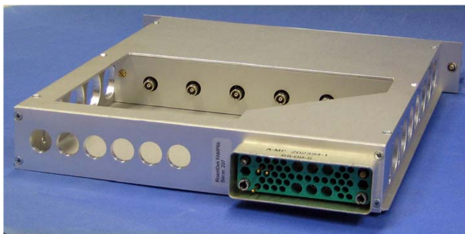
Figure 1: rear panel of FAMP6 (top) with NIM connector and signal inputs, right: front panel of FAMP6 with signal outputs.
