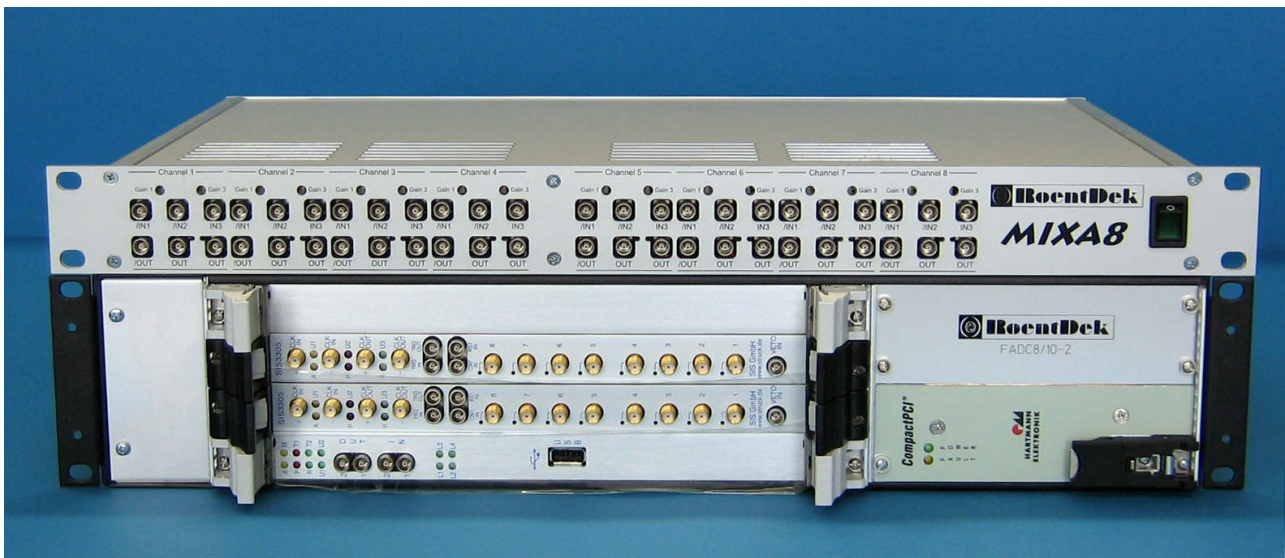
Figure: RoentDek fADC8 module with auxiliary MIXA8 module (here with SMA inputs. LEMO 00 option is also available)
