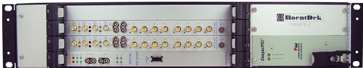
Figures: RoentDek fADC8 module (here fADC8/10-2 ) with two 10 bit ADC units, e.g. for readout of up to two RoentDek HEX anode detectors (here with SMA inputs. LEMO 00 option is also available).
