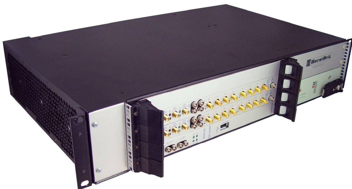
Figures: RoentDek fADC8 module (here fADC8/10-2 ) with two 10 bit ADC units, e.g. for readout of up to two RoentDek HEX anode detectors (here with SMA inputs. LEMO 00 option is also available).
