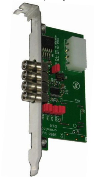
Figure 2.1: External clock module
