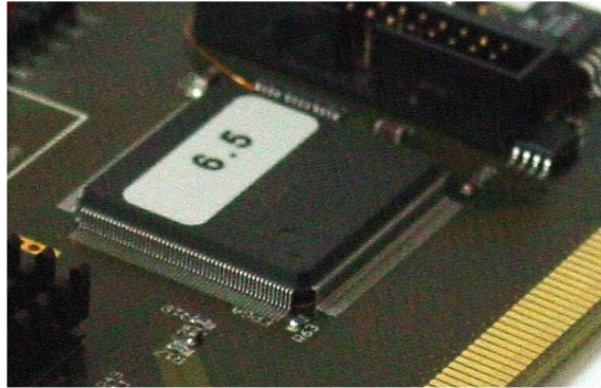
Figure 1.5: The card's serial number located on the PCI-interface chip. The first digit denotes the year of production minus 2000, the second is a unique serial number.
