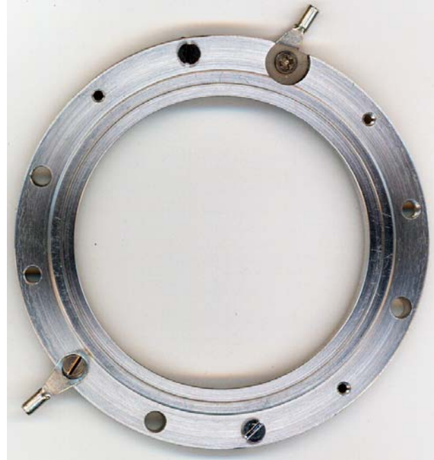
Figure 4: Picture of wMesh40 mounted on a ceramic ring (for mounting options see text below). The cut-out is at the position of MCP front contact. The mesh contact can be made as described for the free-standing meshes or by using the M2 holes as shown here (lower left corner).
